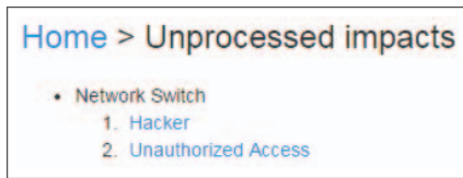
Fig. 2. A list of threats that potentially apply to a component, but for which no impact has been defined yet. A click on one of the links will directly open the appropriate interface to add the corresponding impact.
